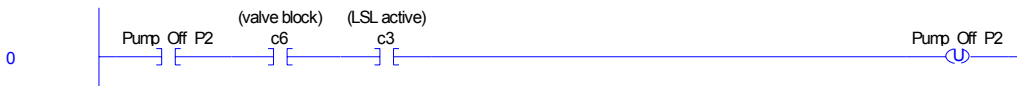
Figure B.3: Tank Control Model Inserted Condition Inputs for t_2 in LLD
