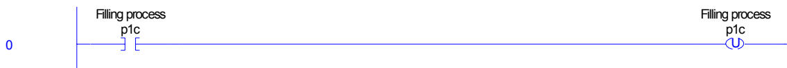
Figure B.7: Tank Control Model Inserted Input Place for t_1^c in LLD
