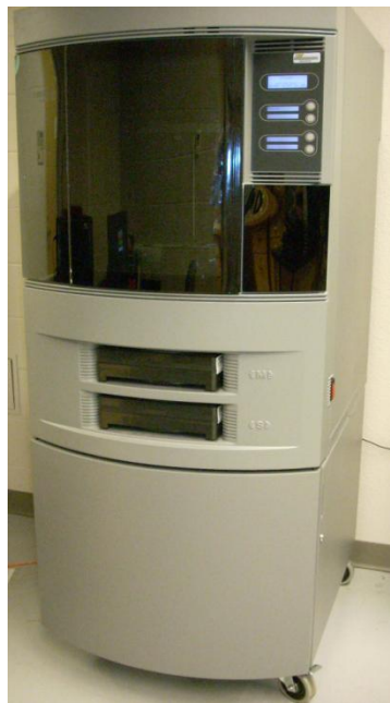
Figure 4.29: Fused deposition modeling (FDM) machine, Dimension SST-768
