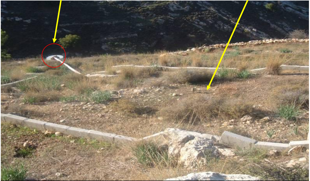
Figure (3) Microcatchment used to measure runoff and sedimentation.
