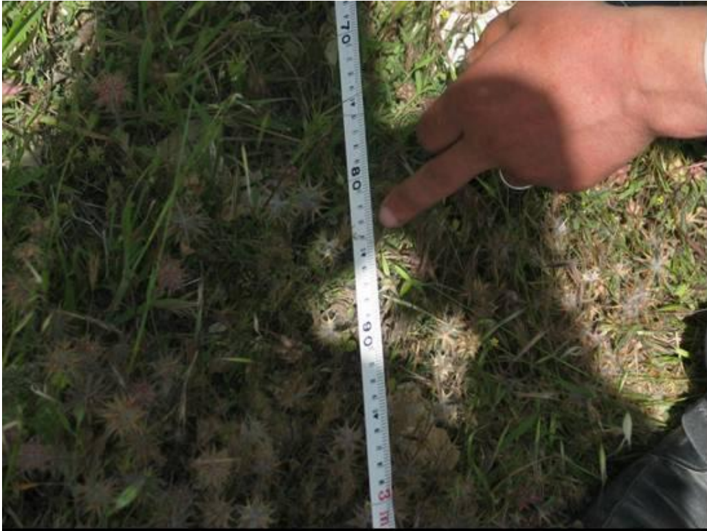
Figure (2) Line intercept method was used to assess ground cover percentage at each treatment.
