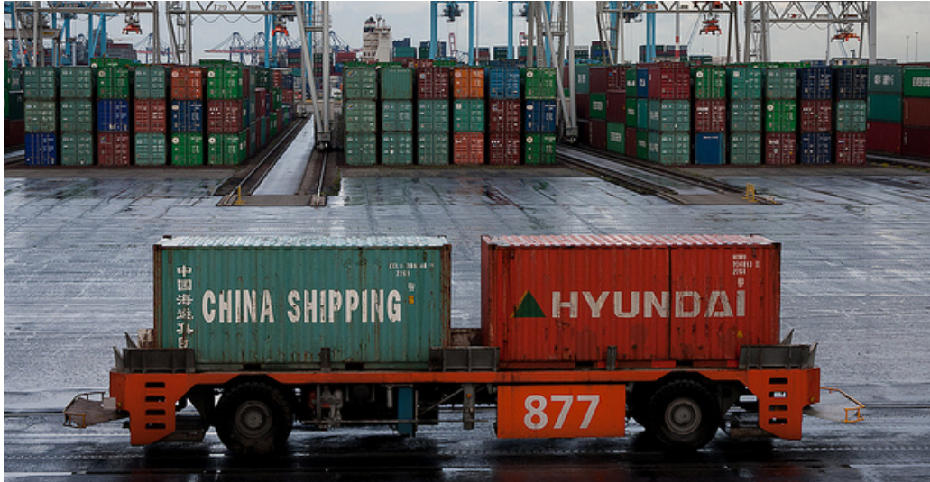
Figure 2.7 An automated guided vehicle
