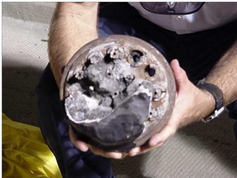
Figure 1.3: Corroded anchorage in Mid Bay Bridge ( www.dot.state.oh.us )
