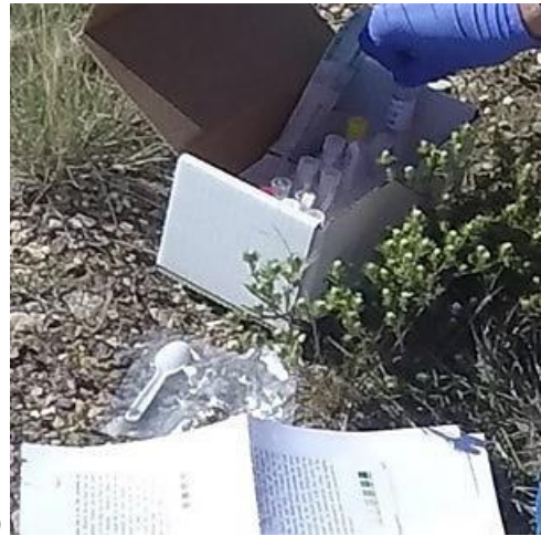
Figure 4.13 Surface-swab testing for chloride and sulfate deposition: (a) test kit by MSES Consultants, Inc.; (b) pole swabbing; and (c) on-site analysis of swab samples.
