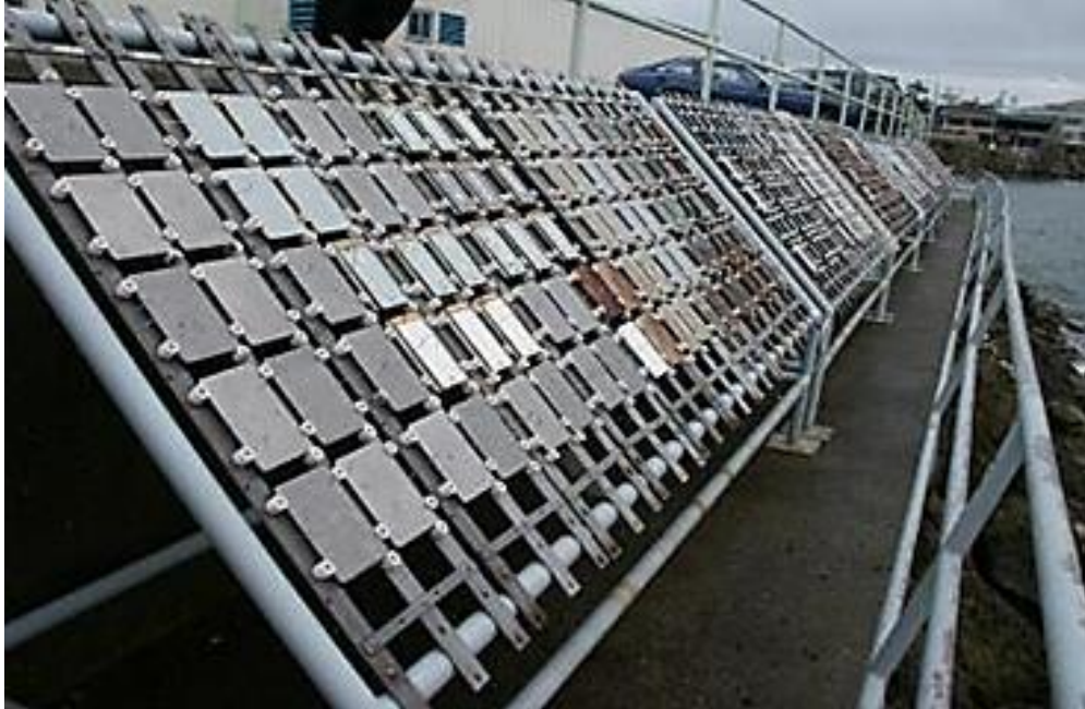
Figure 4.7 Steel panel specimens mounted on inclined rack for corrosion testing in chloride-laden atmosphere (Roberge 2008).
