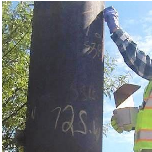
Figure 4.13 Surface-swab testing for chloride and sulfate deposition: (a) test kit by MSES Consultants, Inc.; (b) pole swabbing; and (c) on-site analysis of swab samples.
