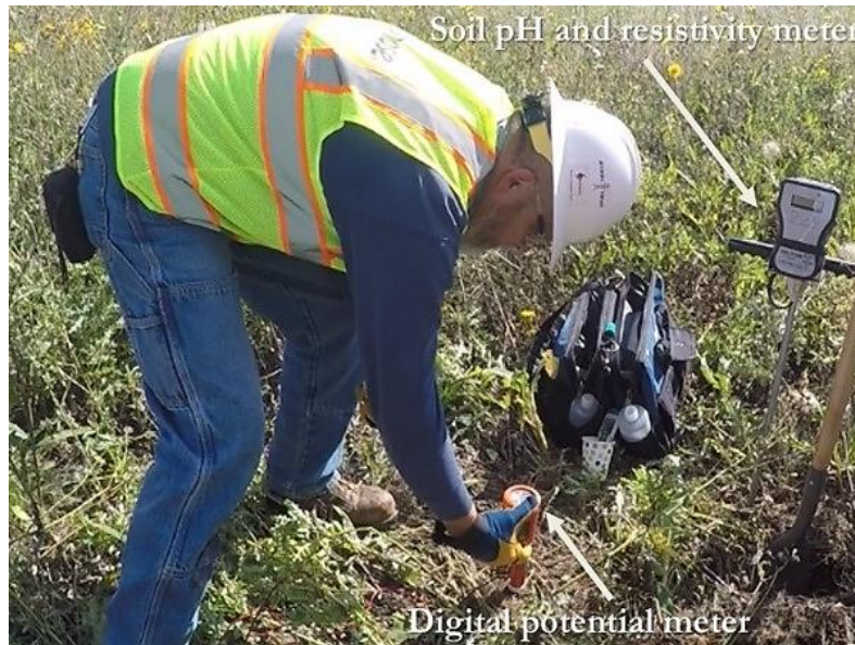
Figure 4.19 Field testing of soil corrosivity.
