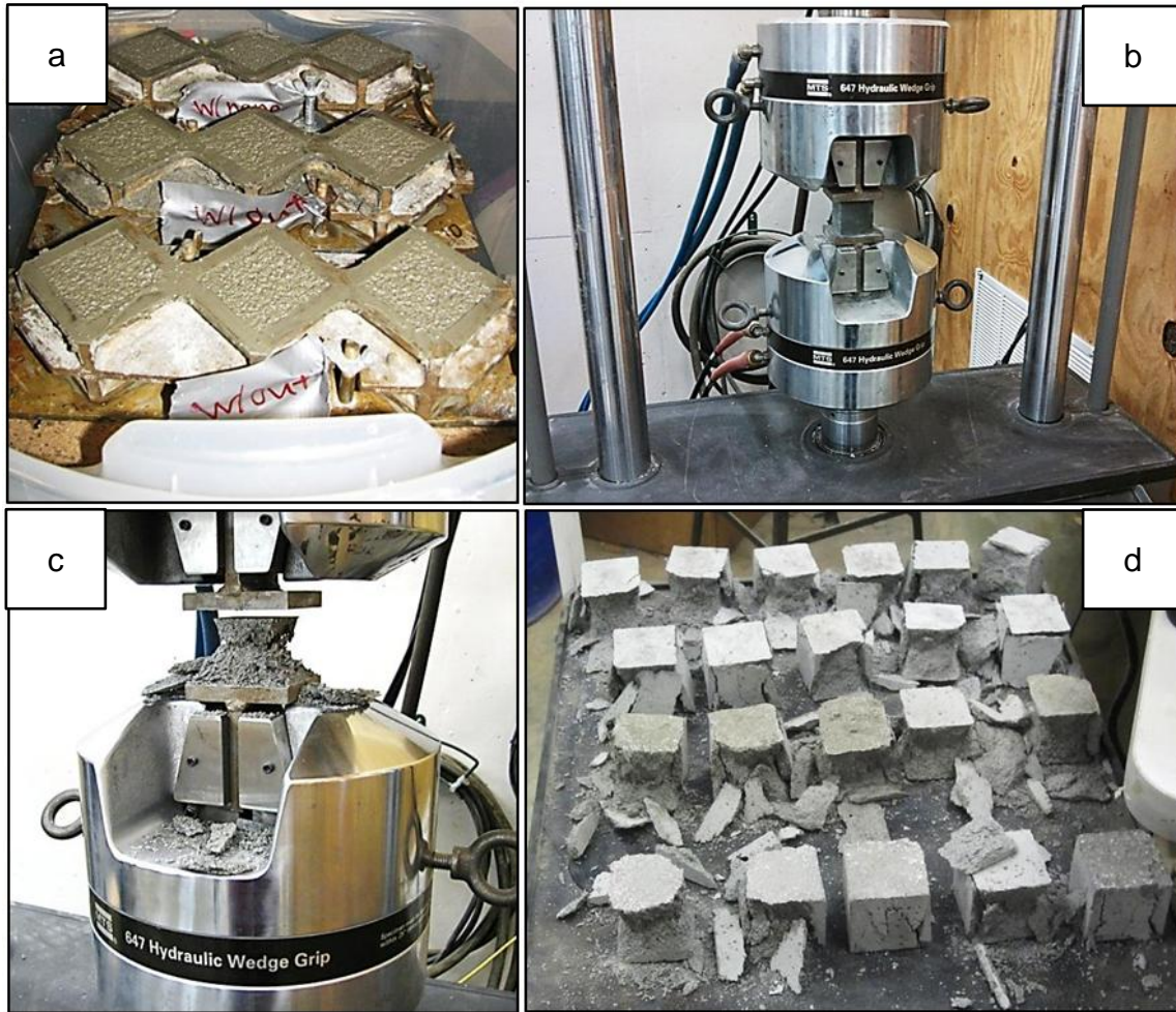
Figure 2.3 - Photographs of compression specimens and tests: (a) moist-curing of cube specimens; (b) cube specimen under compressive load, (c) failed cube specimen, (d) failed specimens
