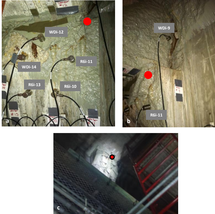
Figure 5.2 Photographs of the crane maintenance area: (a) main sensor grid, (b) close-up of sensor on side of column, and (c) view of main grid from floor level (red dot is at corner).
