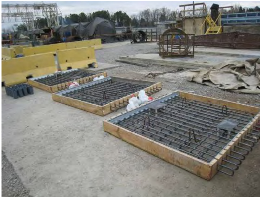
Figure 2.5: Large scale specimens prior to pour (French, et al., 2011)
