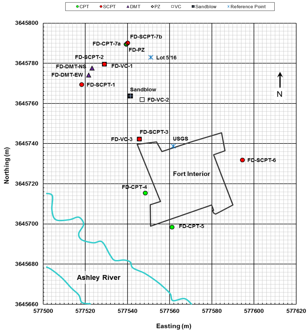
Figure 2.5 Exploration and Test Locations at the Fort Dorchester Site (after Talwani et al. 2011)
