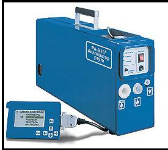
Figure 2. 2: The RA-915+ used by EPA to measure mercury vapor concentration in air.
