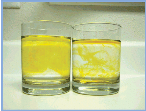
Image 2: Diffusion Molecules diffuse from an area of high concentration to an area of low concentration.
