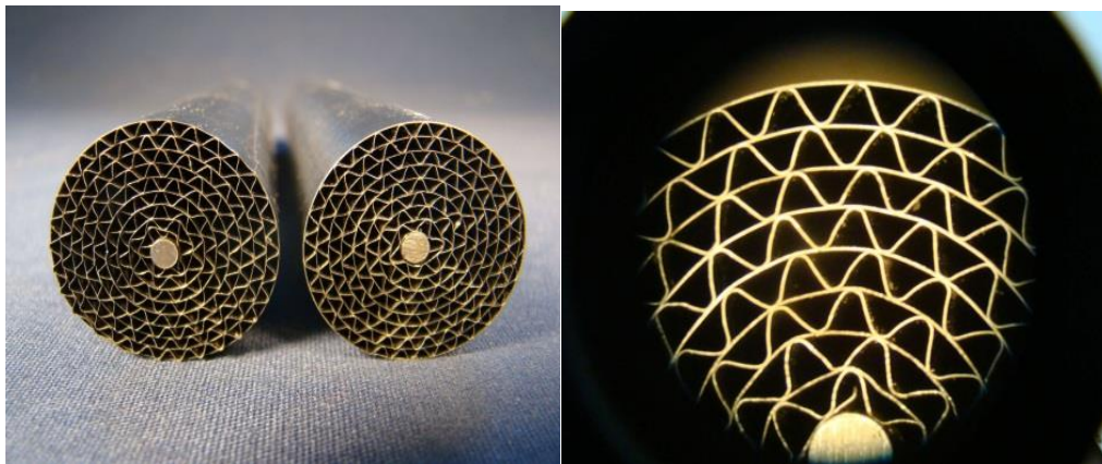
Figure 3.2 Catacel corrugated structures with triangular channels
