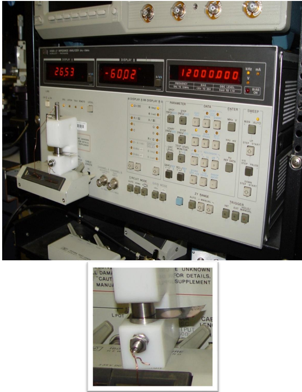
Figure 2.1. Impedance Analyzer (Agilent 4192A LF).
