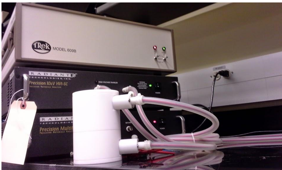
Figure 2.2. From bottom to top; radiant ferroelectric tester, high voltage interface, and high voltage amplifier in a stack.
