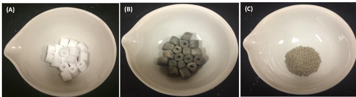
Figure 2.2 Pictures of (A) SA5562 \alpha -Al 2 O 3 rings (B) Ag-Cs-Re-Mo/ \alpha -Al 2 O 3 catalyst (C) sieved Ag-Cs-Re-Mo/ \alpha -Al 2 O 3 catalyst for reaction.
