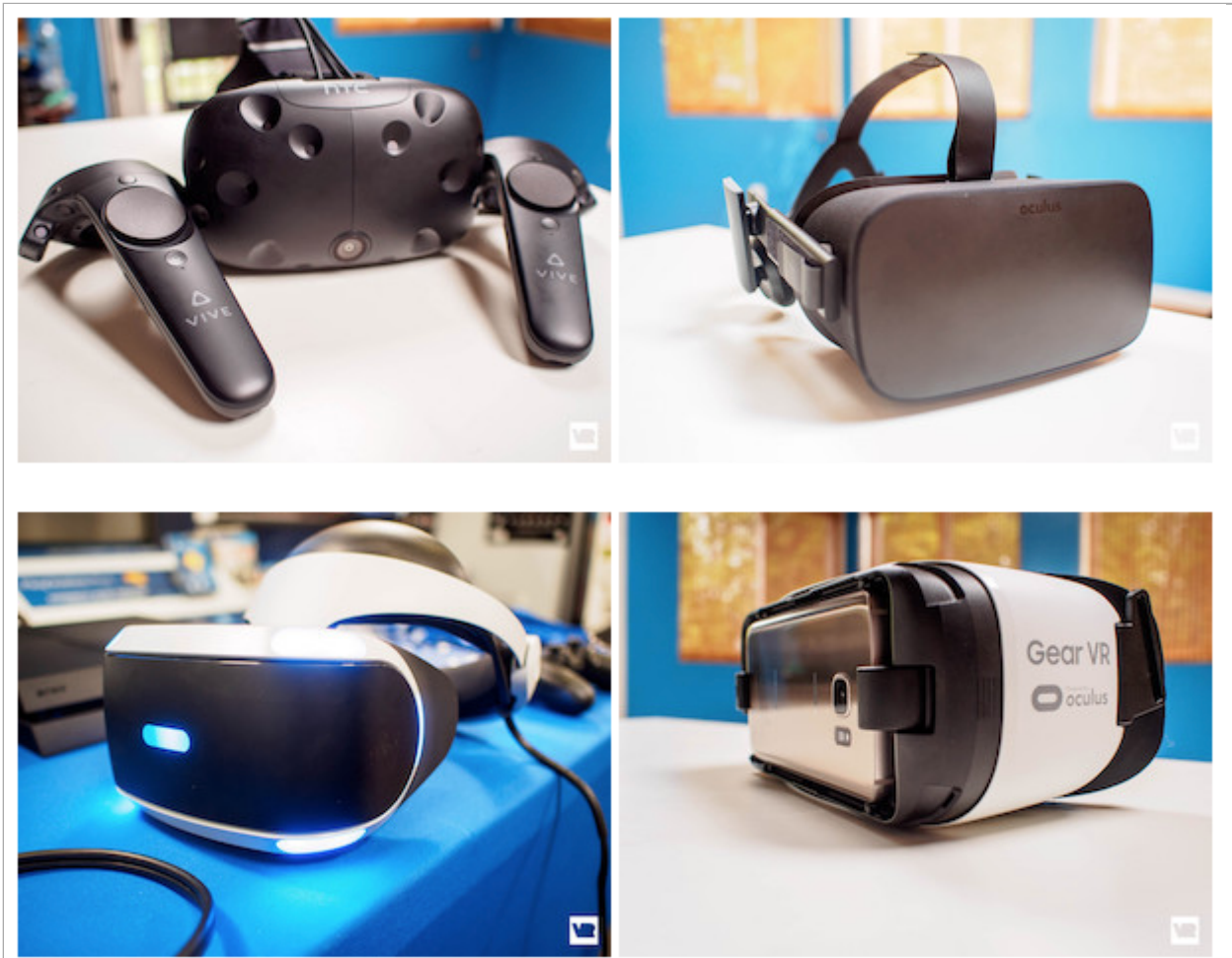
Figure 1. Currently available consumer VR HMD systems. Clockwise from top left: HTC Vive, Oculus Rift, Sony PlayStation VR, Samsung Gear VR.
