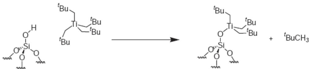
Figure 1.9 Grafting reactions of tetrakisneopentyl titanium on silica [36].
