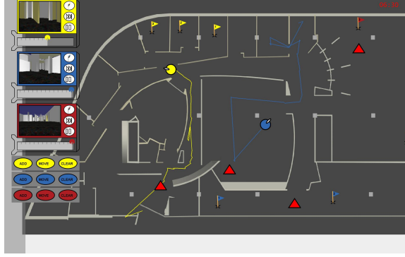
Figure B.2 The Wayfinder application. Visible are vehicles (circles), threats (triangles), waypoints (flags) and control panels (left).
