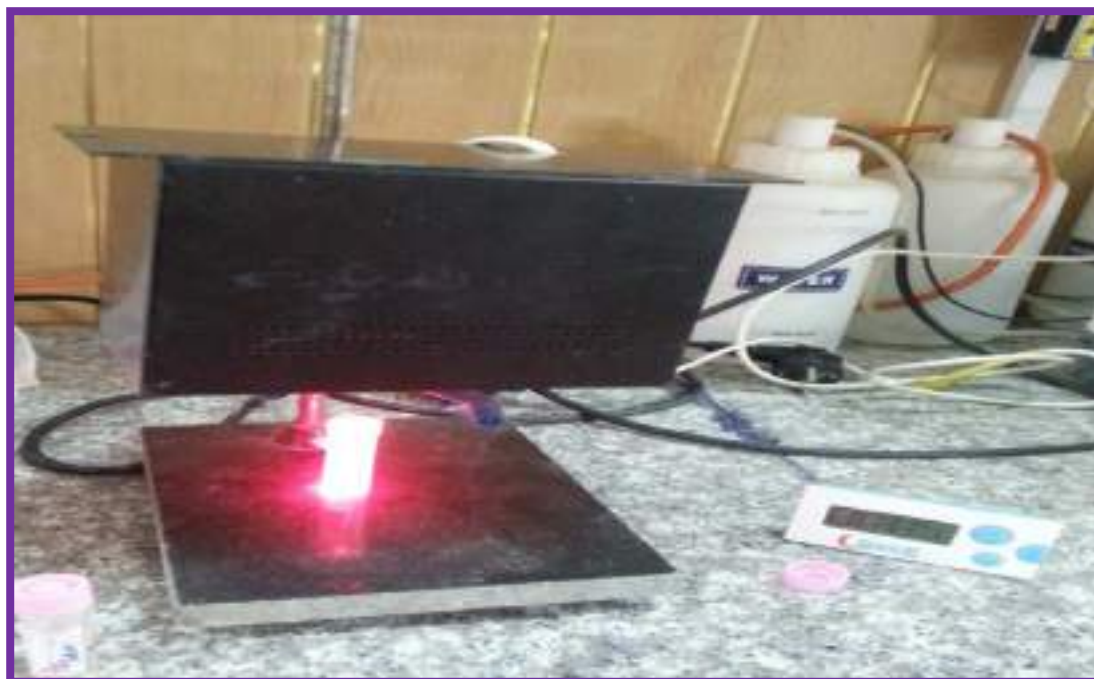
Figure (3-10): Represent a picture for Diode laser with 50 mW.
