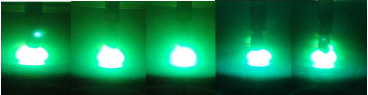
I=62A, V=33.5v, d=10mm \ i=60A, V=32.6v, d=9mm \ i=59A, V=32v, d=8mm \ i=57.9A, V=31.8v, d=7mm \ i=57A, V=31.2v, d=6mm
