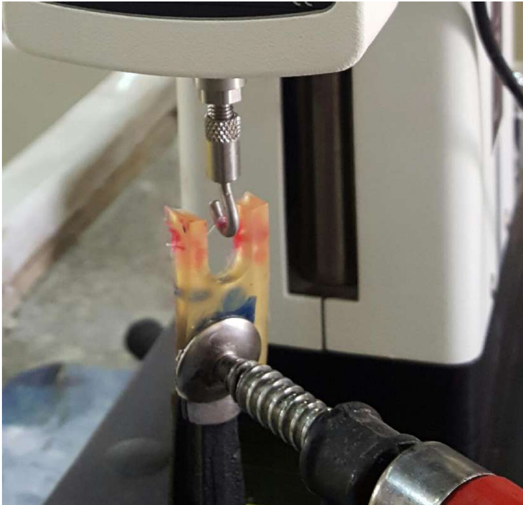
Fig (3-6) U-shape specimen in ESM0301 motorized force tester mark-10
