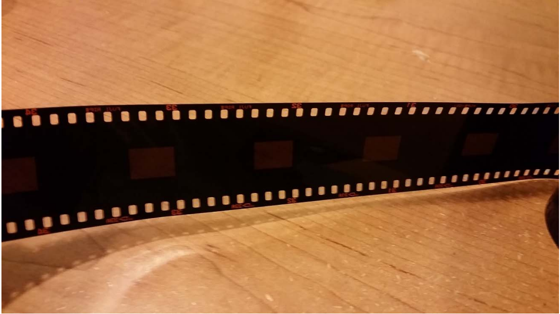
Figure 17 This is an example of a printed mask on 35mm film.
