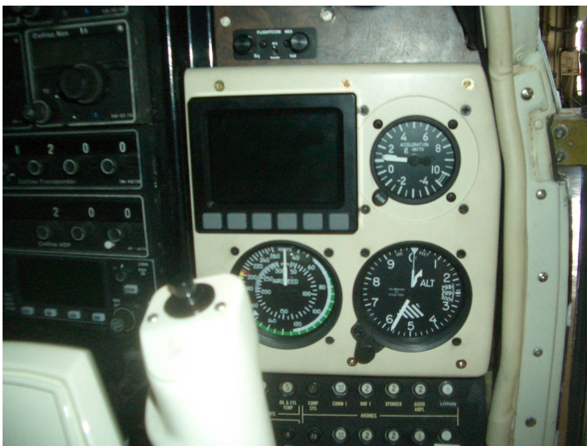
Figure 63 Supplemental instrument panel with Dynon EFIS-D10A installed.
