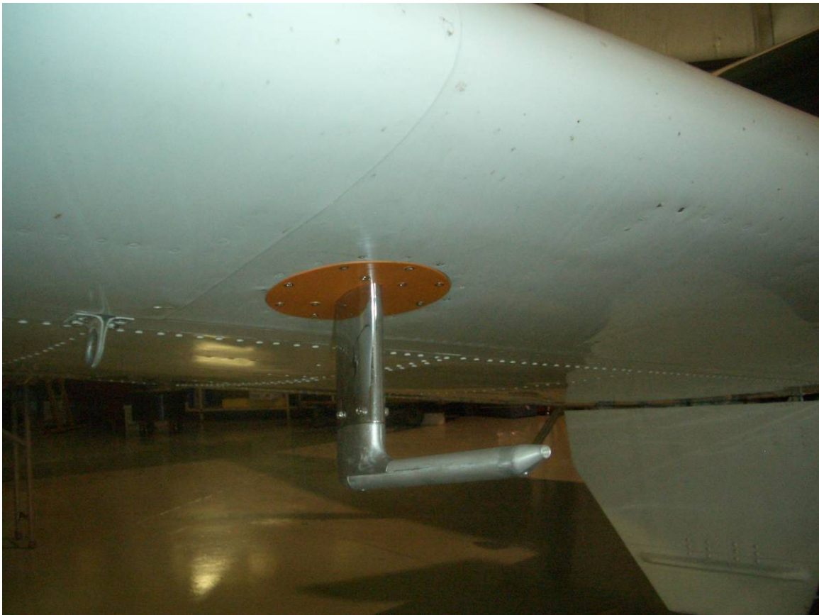
Figure 64 Dynon pitot and angle of attack probe fitted below the right wing.
