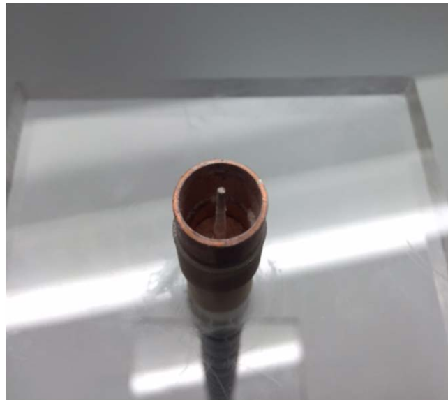
Figure 32. Inner conductor and pulverized mussel shell insulator of the coaxial Tx. line
