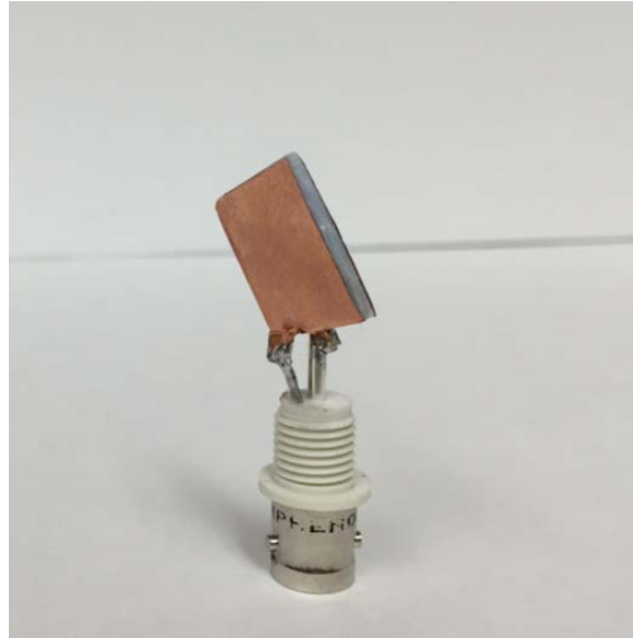
Figure 27. Mussel shell parallel plate capacitor soldered directly to BNC connector
