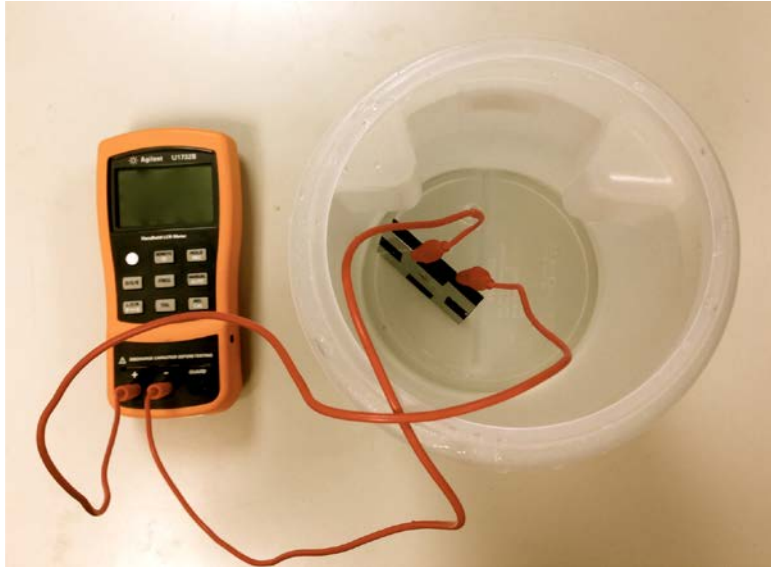
(a) Measurement setting using a portable U1732B Agilent LCR meter.
