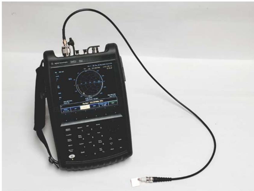
Figure 28. VNA with mussel shell parallel plate capacitor
