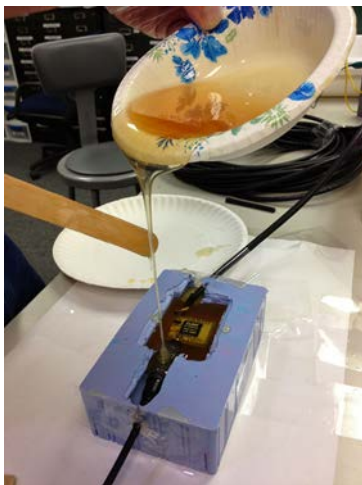
Figure 49. Any type of underwater work with electronic devices such as radios mounted in a circuit board requires significant effort to properly waterproof the equipment.
