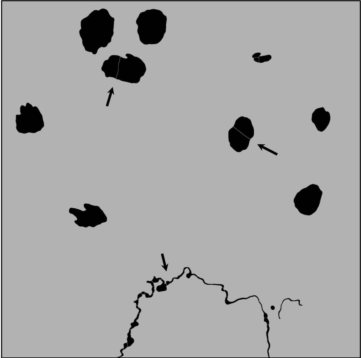
Figure 31 – Mask Of Image With Watershed Algorithm Applied; Mussels Are Segmented Into Multiples Pointed Out By Arrows.
