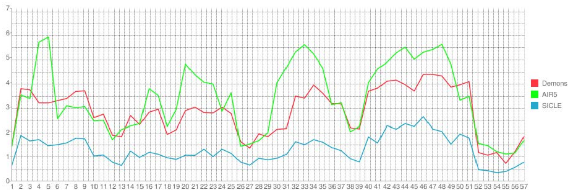
Figure 3.30: Graph of Transitivity Error using second method for 57 ROIs which was computed by averaging TE1 average values for 18 NA0 datasets, computed for 306 transformations from three registration algorithms.
