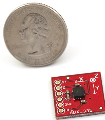
Figure 44. Photograph of the ADXL335 mounted on a breakout board. The accelerometer is used to determine the angle of operation of the microwave rain gauge.
