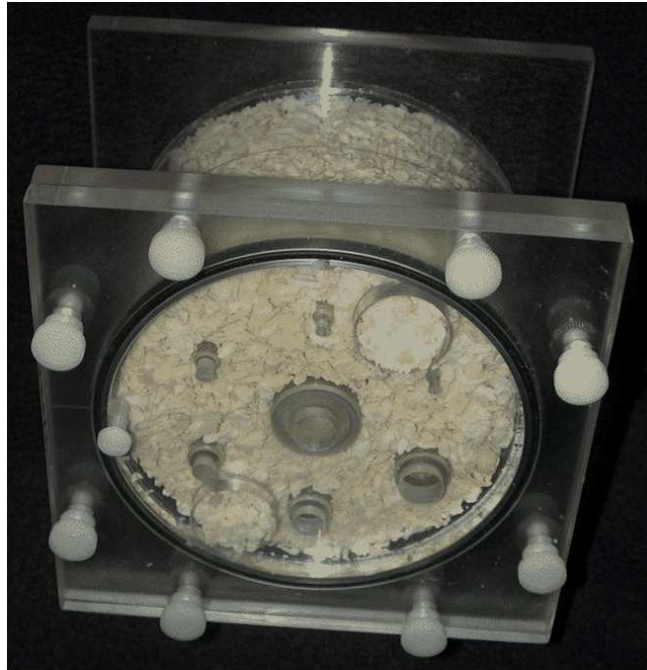
Figure 2.14: The Plexiglas phantom used in the airway measurement accuracy testing
