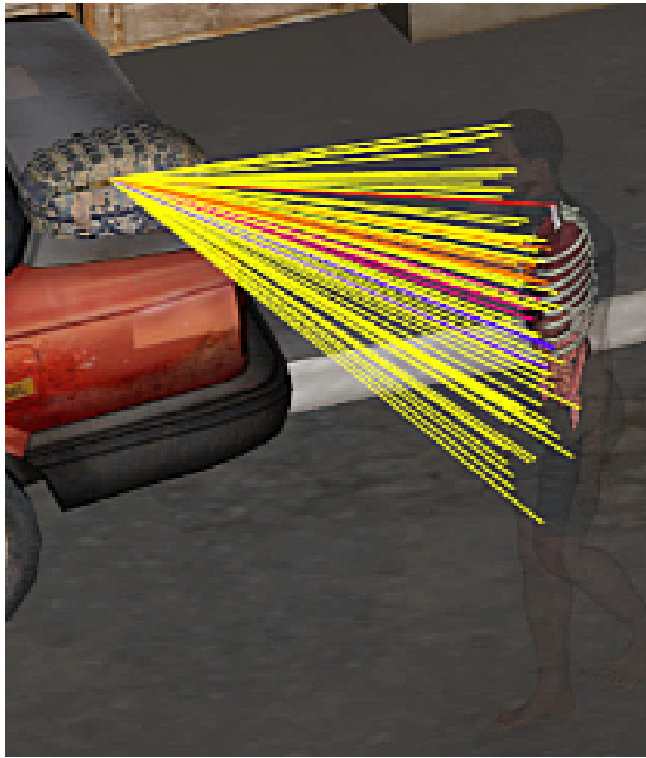
Figure 44: Real time hit-detection and damage score in Santos with each color of the ray indicating a hit of a different body part
