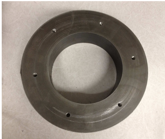
Figure 3.4: Unslotted toroid for core loss measurement
