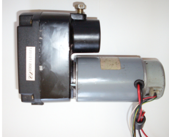
Figure 4.4: Photograph of the chosen DC motor and gear box.
