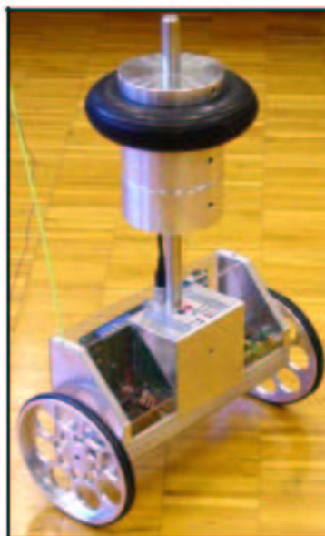
Figure 1.3: Photograph of JOE: A Mobile, Inverted Pendulum.
