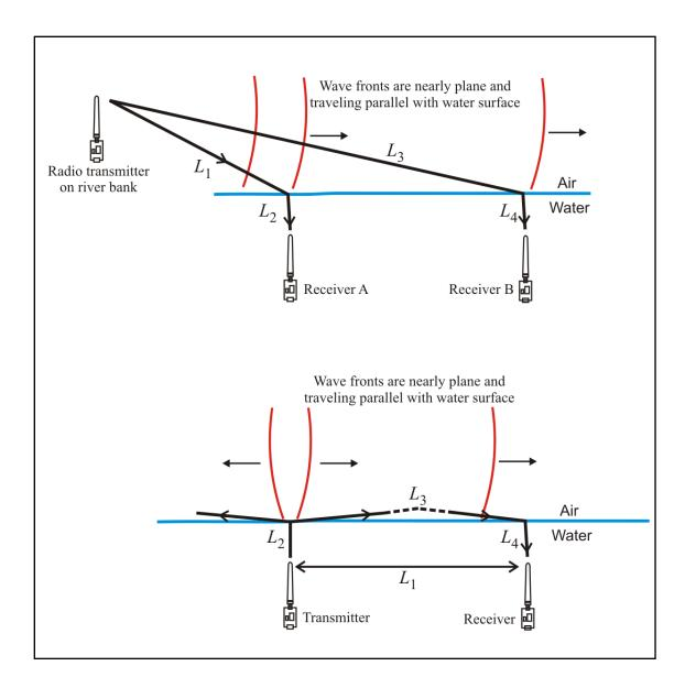
Figure 4 The top figure shows a transmitter on a river bank transmitting to two receivers in a river. The transmitter is far enough so that one can consider the wave fronts and essentially plane and traveling nearly parallel with the water surface. At the surface, some of the radio wave energy is refracted into the water and travels distances  $L_1$  and  $L_2$  to the receivers. The bottom figure shows two radios underwater communication with each other.
