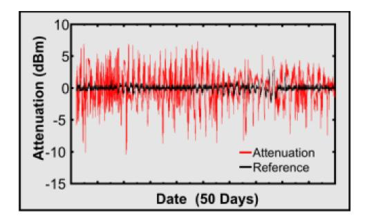
Figure 59 RSSI for links ES3, ES4, and ES5 were averaged for comparison with leaf wetness sensor data. The reference link outside the corn shows much less variation, supporting the hypothesis that the plant moisture modulates RSSI.
