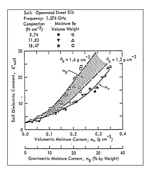
Figure 5 Typical soil dielectric constant at about 1.1 GHz as a function of gravimetric soil moisture  $(m_g)$  and volumetric soil moisture  $(m_v)$  (from Barkeshli, 1985). Note that the dielectric constant show much less scatter when plotted as a function of  $m_v$ .
