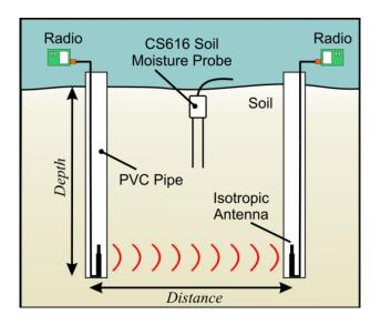
Figure 26 Experimental setup for measuring RSSI as a function of antenna depth and separation distance using XStream radio modules. Antennas were lowered in to PVC tubes that were driven in the ground. Campbell Scientifics' CS616 monitored changes in soil water content.
