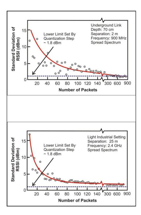
Figure 8 These figures show the how the variance of RSSI values decrease with a number of packets averages. Two cases are shown: one for a 900 MHz underground link, and 2.4-GHz link in a light industrial setting. The figures also show the lower bound, determined by the radio's quantization step size. From the figures it follow that averaging more than about 300 packets (1<sup>st</sup> link) and 80 packets (2<sup>nd</sup> link) does not decrease the variance. However, it does require more power.
