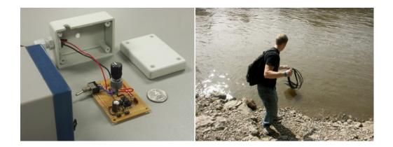
Figure 12 Left: Electronics and enclosure used for making conductivity measurements in freshwater. Right: Nick Sitter deploying the conductivity sensor into the Iowa River by the Stanley Hydraulic Laboratory in Iowa City.
