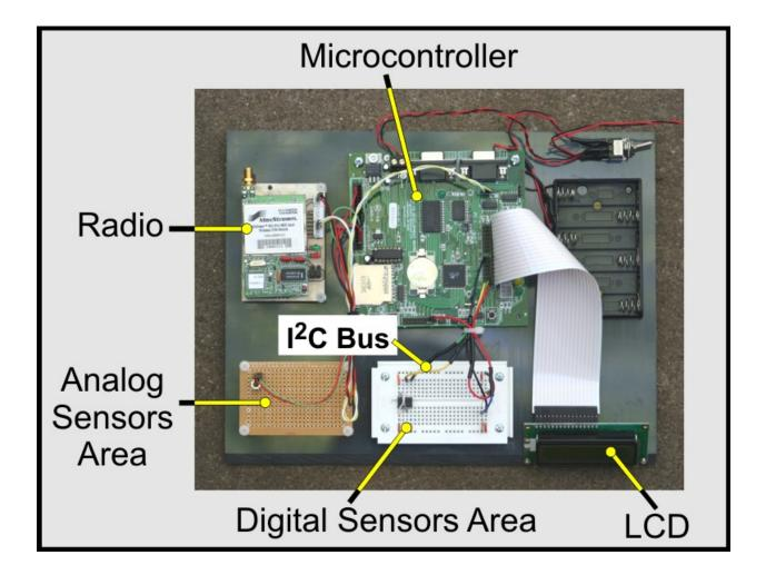
Figure 29 EduMote node used in field experiments and for teaching purposes at The University of Iowa. The EduMote consist of power supply, ATmega128 microcontroller, MaxStream radio, LCD, and sensor area.
