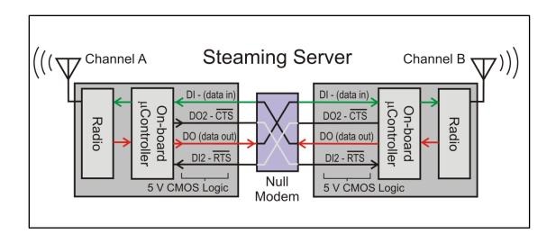
Figure 10 The streaming server consists of two RF modules operating on different channels. The data in lines of both modules are connected to the data out of the opposite module. For example all data received by the module operating on channel A is transmitted out by the module operating on channel B. The channels must be selected as not to be interfering with each other.
