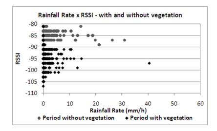
Figure 52 Scatter plot of cell modem RSSI vs. rainfall rate. The data suggests that there appears to be no correlation between rainfall and RSSI of the cell modem.
