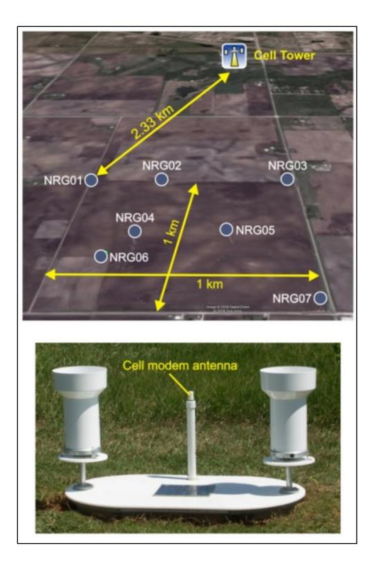
Figure 41 The top panel shows the experimental site at Ames, Iowa, and the bottom panel shows the dual tipping platform that houses a cell modem for relaying data. We observed variations in the cell modem RSSI, which inspired the techniques outlined in this chapter.
