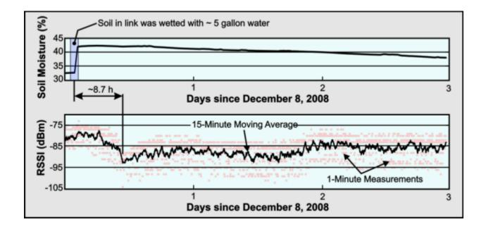
Figure 34 Time-series of RSSI data for link  $R_2 - R_3$  in Path 1 in the prototype WSN. The soil was wetted with ~5 gallons of water shortly after the start of the test. As the water seeps into the soil, the link's attenuation increases (RSSI decreases) and then slowly increases as the soil dries out.
