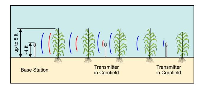
Figure 53 Schematic of experimental concept. Small, low power radios are placed inside a corn field and transmit to a base station outside of the field. Leaf wetness modulates the attenuation through the canopy. The base station records the received signal strength indicator (RSSI) and allows one to infer leaf wetness.
