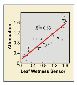
Figure 62 Scatter plot of leaf wetness sensor output voltage versus normalized attenuation of the averaged RF signal for links ES3, ES4, and ES5. A correlation coefficient of  $R^2 = 0.83$  was calculated
