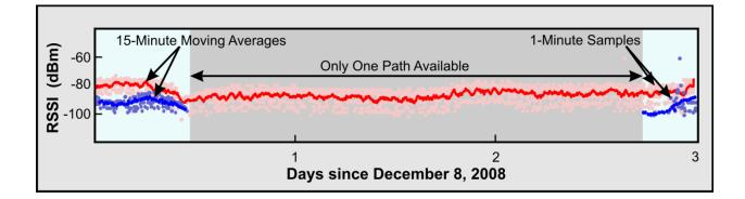
Figure 33 RSSI for a three meter link (blue) and a shorter alternative path (red) are shown for a three day period. As the soil was manually moistened, the longer link began to drop packet and only the alternative route was available for packet routing. Packets were transmitted every two minutes and the dark lines are the five minute moving average of RSSI.
