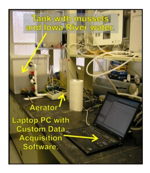
Figure 19 Experimental setup for collecting data of both tethered and untethered intrumented mussels. Mussel gape was sampled at five second intervals for tethered mussels. Mussel gape was sampled at 10 minute intervals for untethered mussels to conserve battery power.
