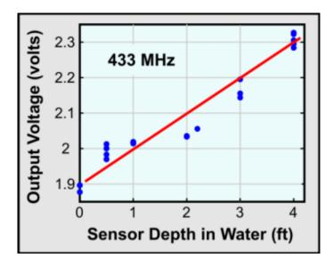
Figure 67 Results from the phase measurement experiment. The data suggest that it is possible to measure water depth by measuring the TOF. Unfortunately results were skewed by the functionality of very off-shelf modules depicted in the thesis.
