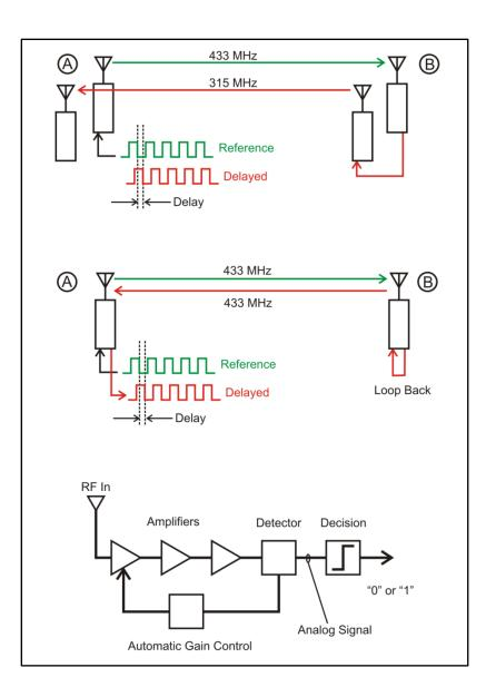
Figure 63 Top is the possible implementation of measuring TOF using a streaming server. Latency is a function of the fixed overhead of the radios and
