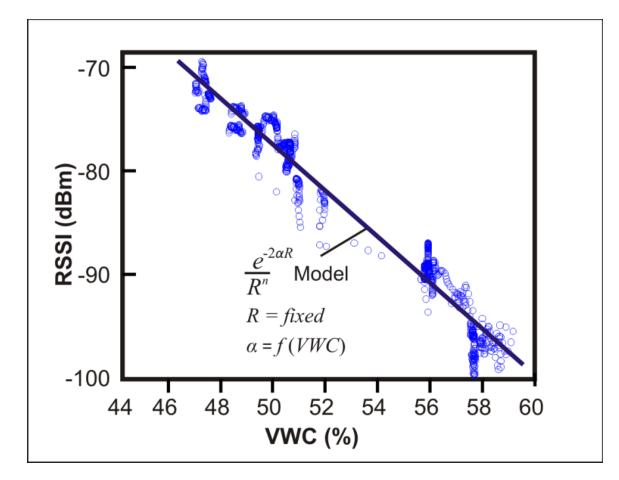
Figure 40 Measured RSSI for links of distance 2.6 m for various VWC. The data follows the model  $e^{-2\alpha R}/R^n$  for fixed distance R and  $\alpha$  is a function of VWC.
