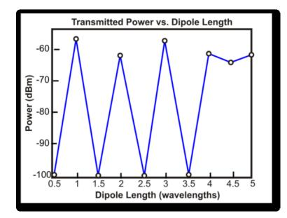
Figure 22 Measured received power as a function of transmitter antenna length for a separation distance of 70 cm in water.
