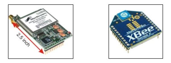
Figure 25 Shown left is the 900-MHz radio, and shown right is the 2.4 GHz radio for the underground communication link feasibility test.
