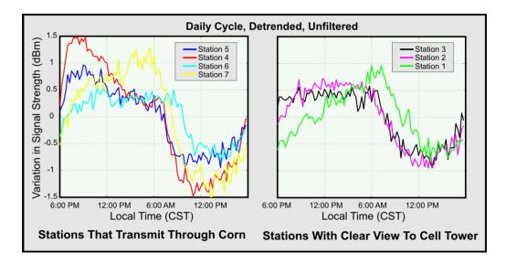
Figure 51 An "average day" RSSI obtained using data stacking. The left plot is for stations that transmit through the corn, while the right plot is for stations that have a clear view to the cell tower.
