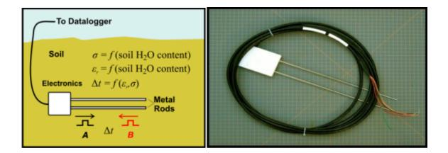
Figure 27 The left panel depicts the principle of operation of TDR-based soil moisture sensors (see text). The right panel is a photograph of CS616 water content reflectometer.
