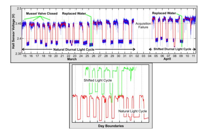
Figure 20 The top panel shows mussel gape data after application of a median filter to remove impulse noise (blue), followed by 5-min zero-phase moving average-type digital filter (red). Low voltages indicate mussel's valve is open. The bottom panel is a phase comparison of mussel gape in natural light diurnal cycle (red) with mussel gape in shifted (approximately 10 hours) diurnal light cycle (green).
