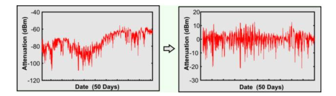
Figure 58 The left plot shows original RSSI data for site ES3 sampled at 2-minute intervals. The right plot is the detrended data averaged to 15-min intervals, and normalized to 0-dBm attenuation.
