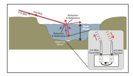
Figure 64 The figure depicts the concept behind round-trip TOF measurements to estimate river stage. A transmitter on the bank transmits on 433-MHz to a streaming server on the bottom of the river. The streaming server echoes back on 315 MHz. The river stage modulates the phase difference between the 433-MHz and 315-MHz signals on the bank. One can easily measure the phase difference and estimate the river stage.
