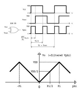
Figure 66 The top panel shows the operation of an XOR gate as a phase detector. The inputs to the XOR gate are square waves at the same frequency  $f_i$ , but not at the same phase. The output of the XOR gate is a series of pulses at frequency  $f_i$ , but the duty cycle is a function of the phase difference between inputs. Low-pass filtering the pulses extracts the average value, giving an output voltage linear with phase difference, as shown in the lower pane.
