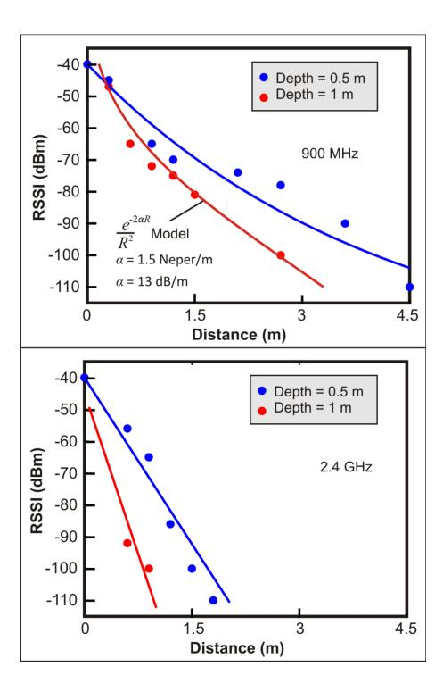
Figure 28 The top panel is RSSI data collected at 900 MHz collected for antennas buried in soil at depths of 0.5 meter in blue and depths of one meter in red for various separation distances. The model is also shown for data collected at a depth of 1 m. The bottom panel shows 2.4 GHz RSSI data collected for antennas buried in soil at depths of 0.5 and one meter for various separation distances. Lines shown are linear approximations for reference only since attenuation of collected data was high.
