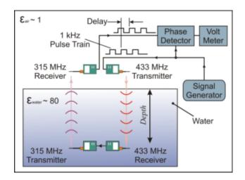
Figure 65 EM waves propagate at ~ 30 ns/m in water. The delay between received- and transmitted pulse trains are  $t_1 + 30 \times Depth$  (ns), where  $t_1$  represents the latencies of the radios, time-of flight through air, electronics, etc.
