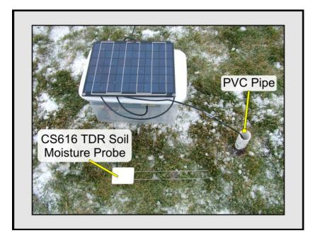
Figure 31 An EduMote, which The University of Iowa uses for laboratory exercises in WSNs, inside its enclosure. I used EduMotes to build the underground WSN. Rather than burying the whole node, we only burry the antennas. Soil moisture was also monitored in between links.
