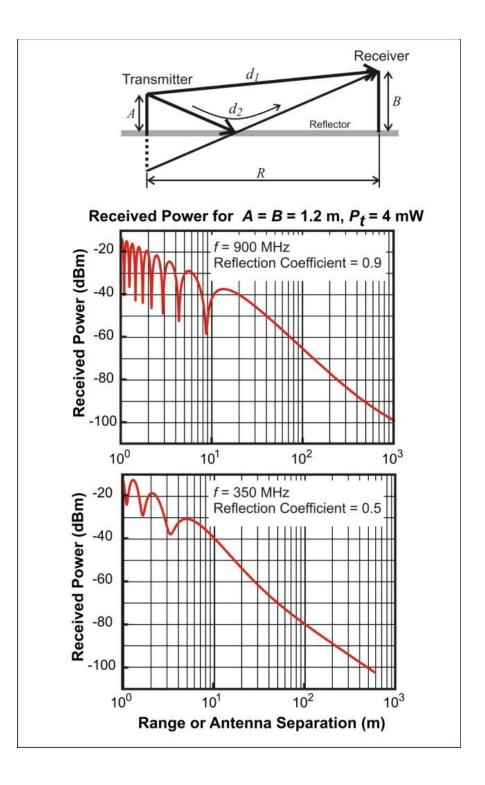
Figure 7 Two-path multipath. The top figure shows a transmitter and receiver at heights A and B above a partially-reflecting plane, separated by a distance R. The path lengths  $d_1$  and  $d_2$  are such that the attenuation is of the same order. However, phase differences can lead to constructive and destructive interference. The middle and bottom figures are examples of such multipath effects.
