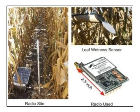
Figure 56 The radio antennas were installed in the center of the cornrows at about half of canopy height. Leaf wetness sensors were installed at one third and two-thirds canopy height. 2.4 GHz RF modules provided the links for making RSSI measurements.
