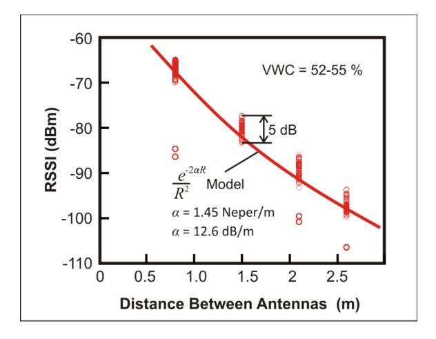
Figure 39 Measured RSSI for all possible links at four fixed distances at near a constant volumetric water content of soil of  $52 \rightarrow 55\%$ . The data follows the simple model with  $\alpha = -18.78 \text{ dB/m}$ .
