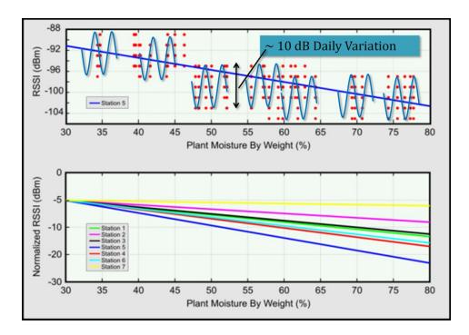
Figure 47 The top plot shows RSSI as a function of plant water content for Station 5. The bottom plot shows normalized linear fits for all stations. Surprisingly, Station 7, which transmits through the longest path of corn, shows the least variation of plant water content.
