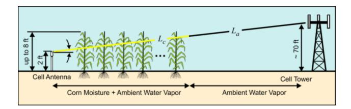
Figure 44 Cell modems in the rain gauge network at the experimental site in Ames transmitted through a combination of corn and air. Antennas are located in the lower one fourth of the mature plant height.
