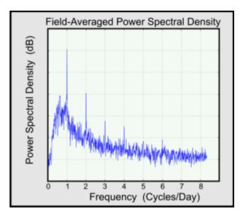
Figure 48 Average (for all stations) power spectral density of RSSI. One can clearly observe a spike at 1 cycle/day, indicating a diurnal cycle in the RSSI. This is consistent with results from Empirical Mode Decomposition (EMD) and Data Stacking, see below.
