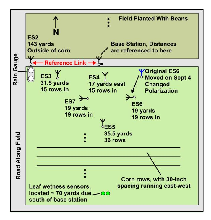
Figure 54 Locations of six RF nodes and base station collocated with rain gauge and leaf wetness sensors in the field in Ames. Node ES02 was used as a control and had an unobstructed view of the base station, all other nodes were located within the canopy.
