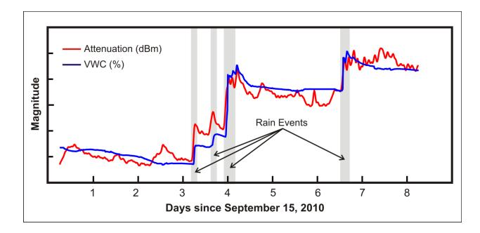
Figure 38 Normalized time series of underground link RSSI (red) and soil moisture data (blue), collected over a nine day period in mid-September 2010. Soil moisture probes were installed to measure water content in the top 30 cm of soil. Radio antennas were buried at a depth of 60 cm. During this period there were four rain events that altered soil moisture content. As the water content of soil moisture increased the attenuation of the RF signal also increased.
