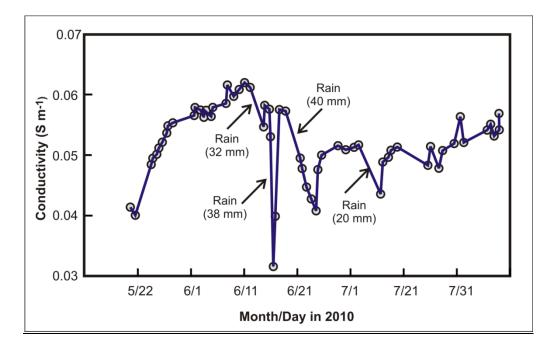
Figure 13 Data collected for Iowa River conductivity from May 21, 2010 until July 31, 2010. Measurements were made twice a day at 8 am and 3 pm local time. A decrease in conductivity is observed after rain events with the influx of distilled water followed increases in conductivity as this water flows downstream. Conductivity during this period ranged from 0.03 to 0.063 S/m.
