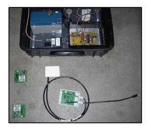
Figure 36 Components used to validate RSSI measurements in making soil moisture measurements. Top: the custom data-logger with cell modem used to collect soil moisture and soil temperature to be transmitted back to The University of Iowa. Lower left: is pair of XStream RF modules with support electronics used for measuring RSSI. Lower right: TDR probe with support electronics used in making VWC estimations.
