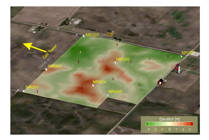
Figure 42 Gauges NRG01, NRG02 and NRG03 are in the flat part of the field with unobstructed views of the cell tower. Gauges NRG04, NRG05 and NRG06 were located on the opposite side of a hill from the tower and NRG07 is located in a depression in the southeast corner of the field. The topography between the deployment field and cell tower was relatively flat.
