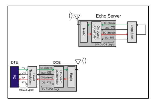
Figure 9 Echo servers are used in several experiments throughout this thesis primarily for range testing. The echo server is exactly what the name implies, all data received from the data communication equipment is sent back. The data out of the RF module is tied directly back to the data in of the module. All communications that are received and forwarded to the data out line are feed back into the data in line and transmitted.
