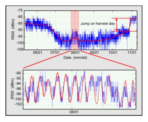
Figure 43 The top plot shows RSSI time series for Station 7. One can clearly observe a longterm decrease, and then a gradual increase in the received radio signal. On the day the corn was harvested, the average RSSI jumped 10 dBm. Other stations showed similar behavior. The bottom plot is an exploded view of time series plot that suggests that a diurnal cycle in the RSSI signal may be present as well (red line, drawn in by hand).
