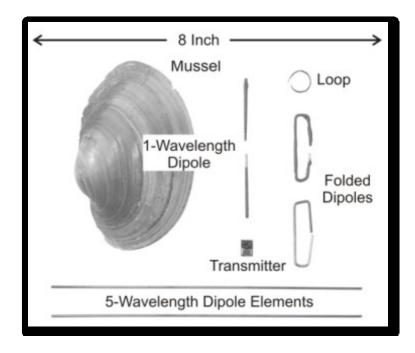
Figure 23 The antennas tested for underwater RF mussel applications at a frequency of 433 MHz.
