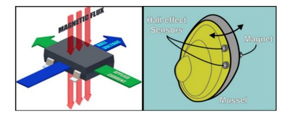
Figure 15 The left panel depicts the Hall-effect, which is the generation of a voltage across a conductor in a perpendicular magnetic field. There are Hall-effect ICs on the market that integrates a Hall sensor with an amplifier and signal conditioning. The right panel shows how we attach a Hall-effect sensor and a small magnet to monitor mussel gape.
