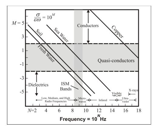
Figure 2 Ratio of  $\sigma/(\omega\epsilon)$  for some common media, including freshwater and soil, which are of interest in this thesis. The figure also shows the range of ISM and cellular communication frequencies. (from Krauss and Felisch 1999). An important conclusion from the figure is that one can consider freshwater and soil as lossy dielectrics at these frequencies.
