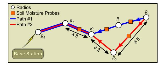
Figure 30 Schematic of proof-of-concept buried WSN. Packets are routed from R0 to R4 via Path #1 as well as Path #2. Packets' payloads are the links' RSSI measures. R4 transmits the payloads to the base station above ground.
