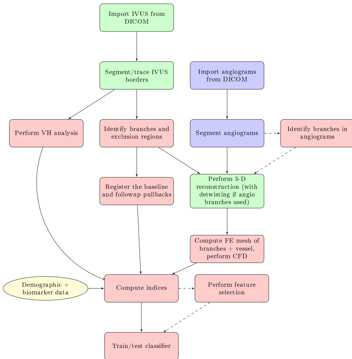
Figure 1.1: Data processing flowchart. Red blocks are new work, blue blocks are untouched preexisting work, green are old software that was extensively modified. Dotted lines indicate alternative paths.
