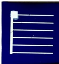
Figure 20. One of the fabricated Si solar cells with a DAR SiN_x coating. This particular cell had an efficiency of 7.49%.
