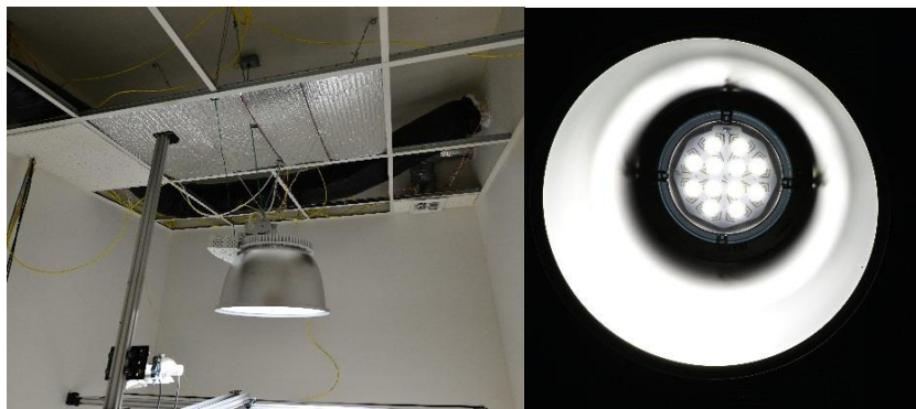
Figure 7-4 Cone-Shape High-Bay with Reflector
