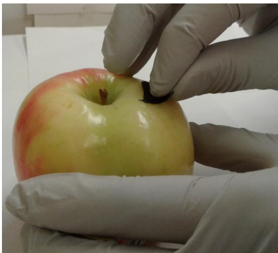
Figure 7.8 Wiping the contaminated area on an apple's skin by carbon cloth electrodeposited with Au for SERS detection of paraoxon
