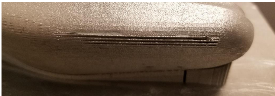
Figure 19: Peeling Contour pass
