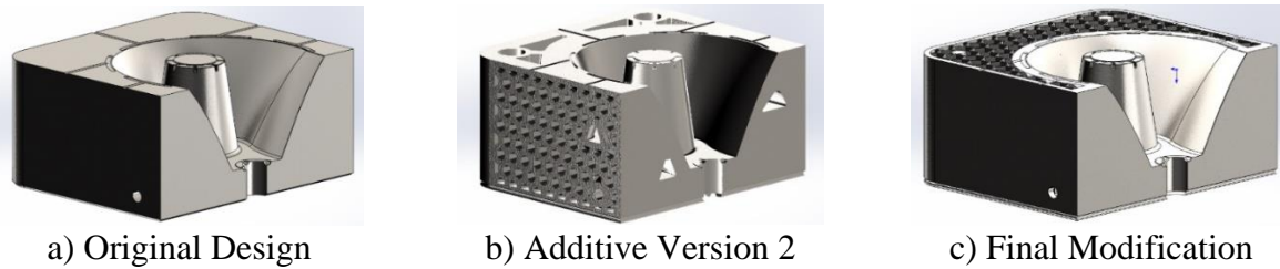
Figure 33: Development progression for injection tooling modifications.
