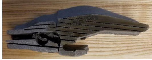
Figure 14: Reducing post-processing by utilizing breakable supports
