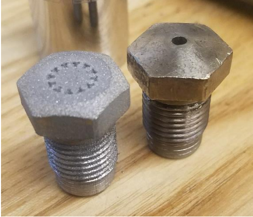
Comparison of additive vs. original nozzle design.
