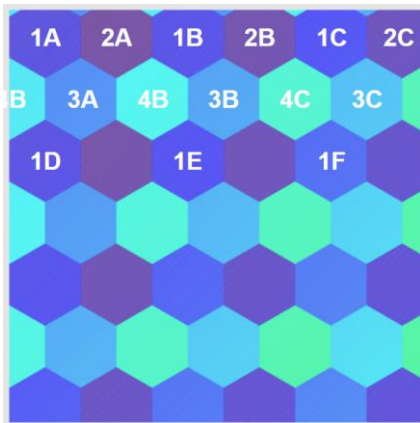
Figure 30: Hex infill pattern with pattern sequence
