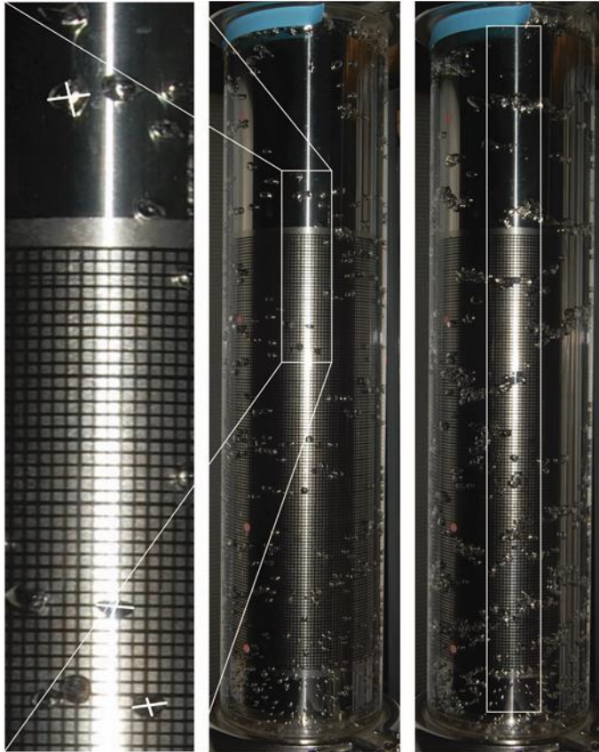
Figure 2.2 Sample bubble images including the measuring grid. Left: magnified view of bubble measurement zone / middle: 300 rpm - 0.235 vvm / Right: 500 rpm - 0.705 vvm; white rectangle depicts the complete bubble measurement area.
