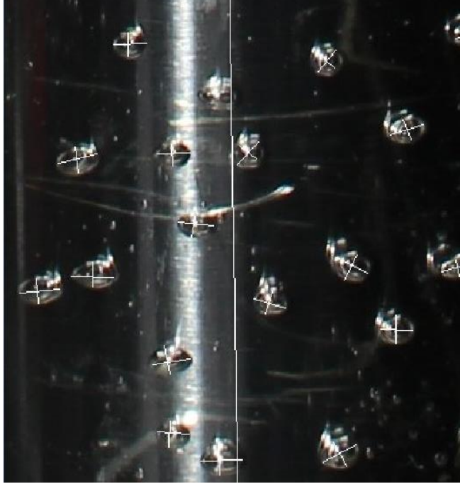
Figure 3.3 Sample bubble image showing major and minor axis measurements.
