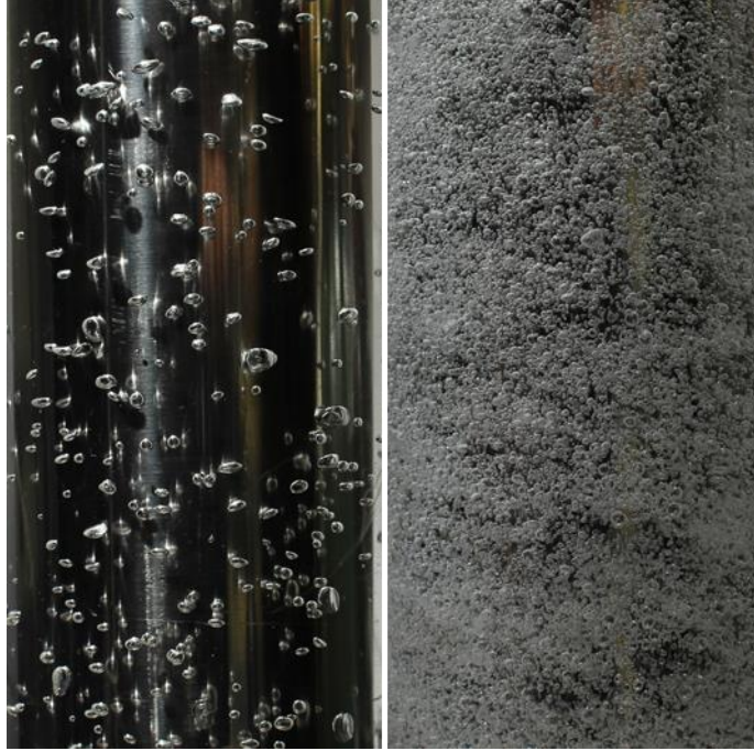
Figure 3.2 Sample bubble images in reactor. Left: Using sparger stone in absence of alcohol / Right: Using sparger stone in presence of alcohol.
