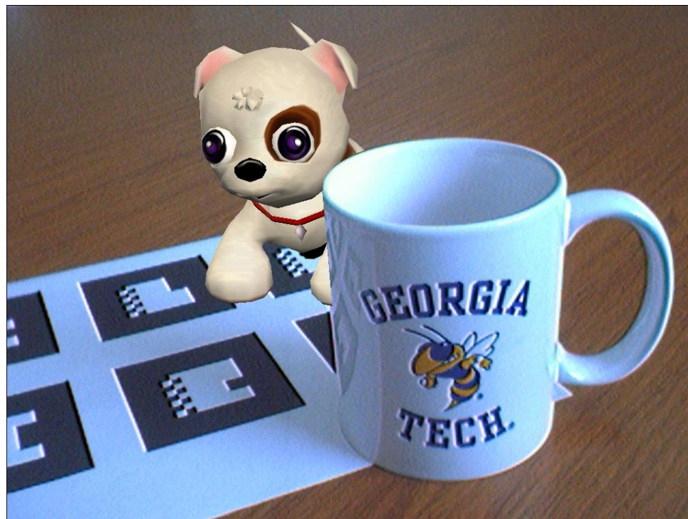
Figure 12. Example of occlusion cues used to provide depth. The virtual dog looks like it is behind the cup (courtesy Blair Macintyre).
