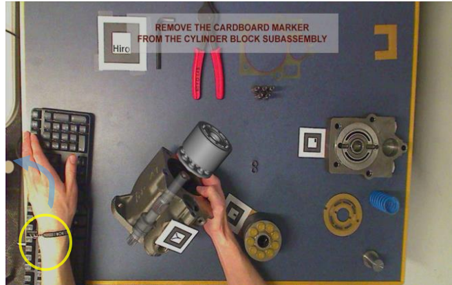
Figure 18. Augmented reality system to aid user in assembling a pump. Textual instructions are provided on top while a virtual demonstration is presented [10]
