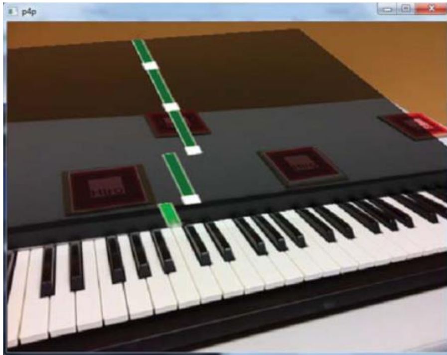
Figure 6. AR viewer used to teach the piano [42]. AR Toolkit markers are used to register the virtual keys with the real keys.
