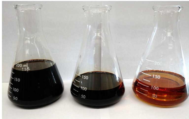
Figure 12. Acetone-free bio-oil from SEP-4 (left) is fed into the bio-oil fractionation system which separates the feed into a raffinate (center) and distillate (right), otherwise referred to as heavy bio-oil and medium oil, respectively.
