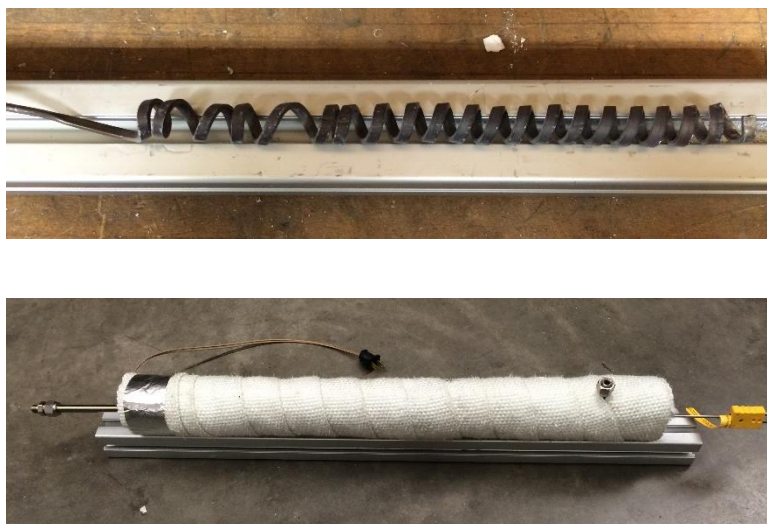
Figure 3.1.2: Heating units, including heating coil (top) and heated flow tube (bottom).
