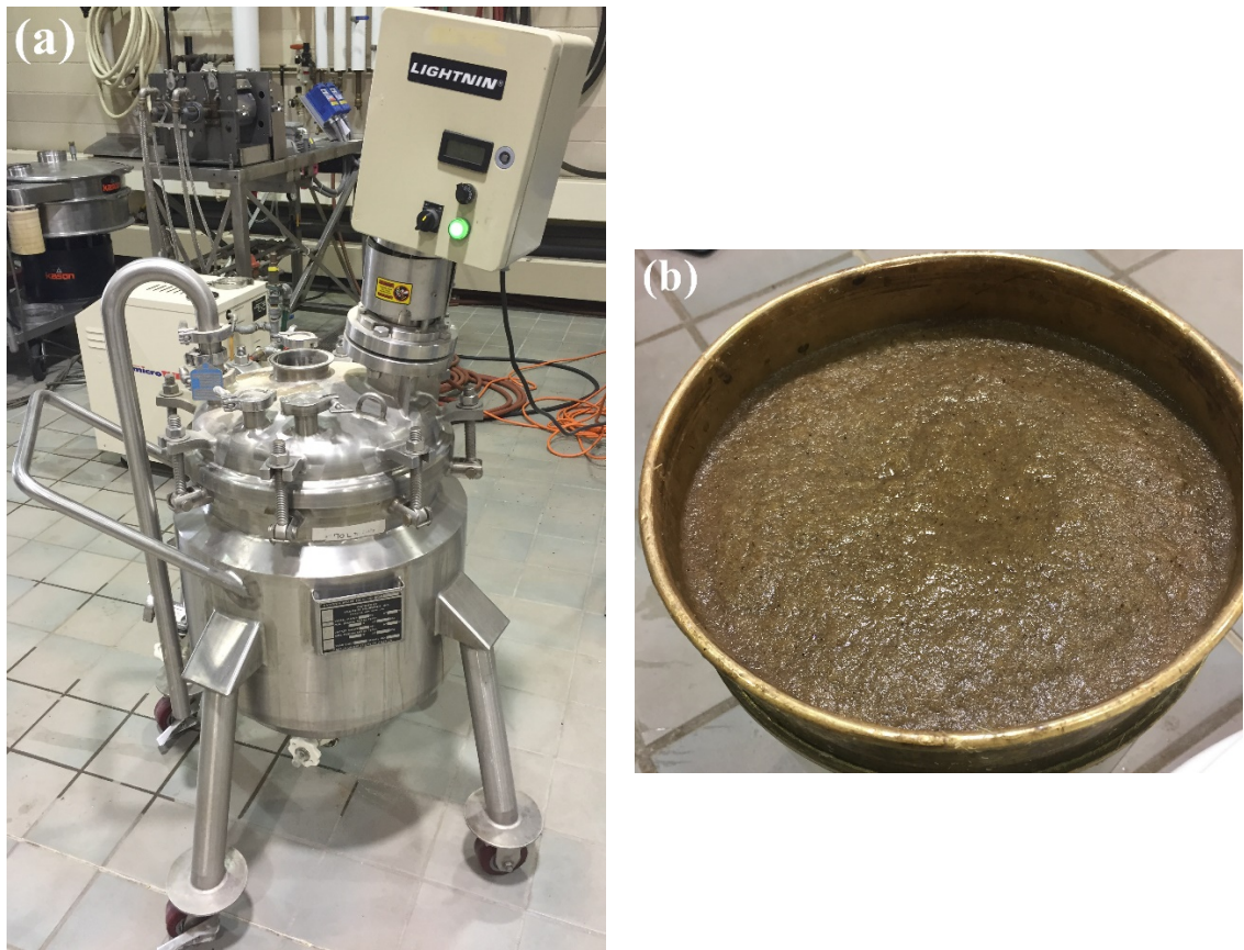
Figure 1. Photos of (a) Feldmeier 70-liter tank and (b) agave fiber during the wash treatment
