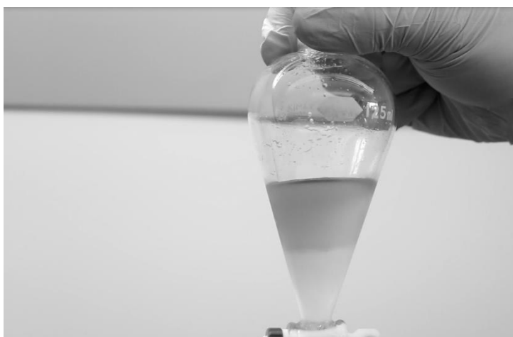
Figure 2. Heptanoic acid extraction of SF5. The topmost layer is heptanoic acid with the extracted organic portion, the bottom layer is immiscible material, comprised primarily of water.
