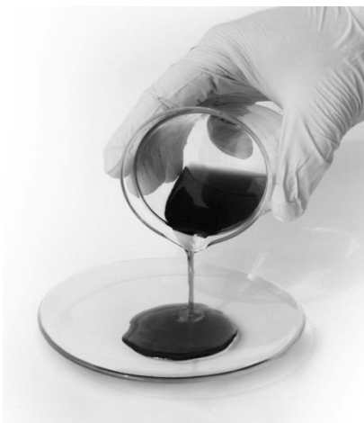
Figure 1. Condensed pyrolytic sugar syrup. Its consistency is similar to food-grade maple syrup that is reddish-orange in color.
