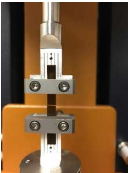
Figure 29. Example of mechanical property test by DHR
