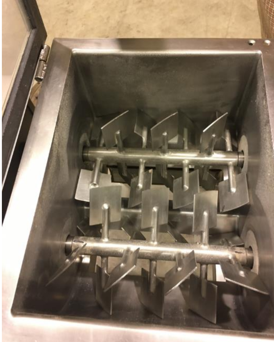
Figure 10: 14,200 cc paddle mixer for biomass acid infusion.
