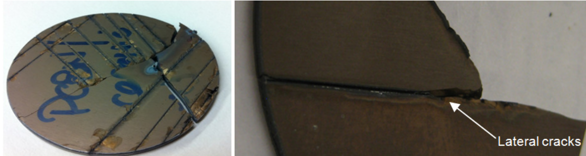
Figure 45: On the left, LWJ on PCBN blank with thick carbide substrate where extensive lateral cracks can be observed. On the right, a complete straight cut of PCBN blank with thin carbide substrate where the cut was controlled for half inch then become uncontrolled and lateral cracks start to appear from the built up temperature in the carbide substrate.
