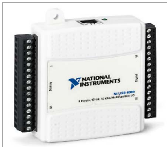
Figure 4.2. National Instruments USB-6009 DAQ
