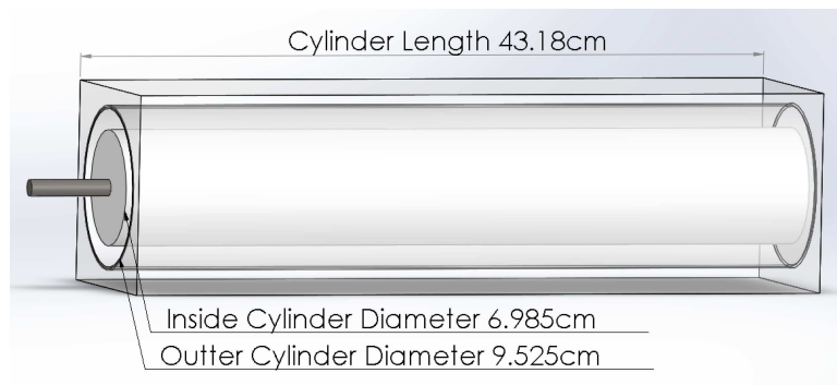
Figure 2.2 Apparatus of experiment: Cylinder Length: 43.18\text{cm} ; Inside Cylinder Diameter: 6.985\text{cm} ; Outside Cylinder Diameter: 9.525\text{cm}
