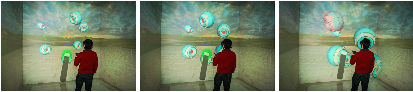
Figure 5.3. Experimental setup with six spheres. Left, the sphere starting positions, middle the spheres approximately at their controlled positions, right the spheres after the goal sphere gets highlighted. The green sphere represents sph_0 .
