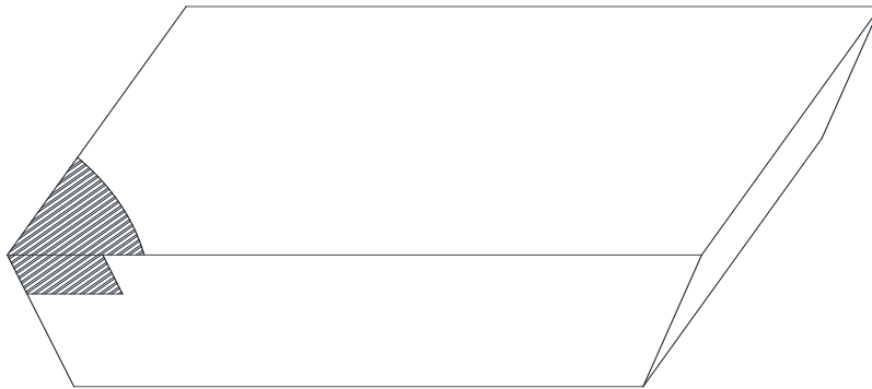
Figure 5.1 Schematic of nanodiamond powders doped in carbide insert tool
